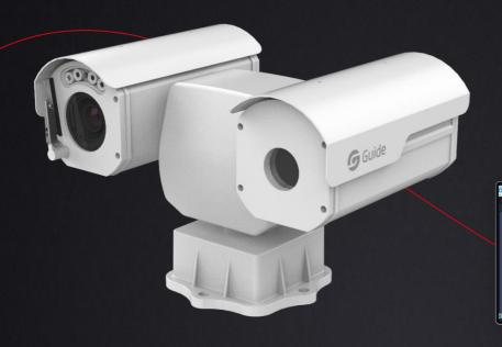
DS60xxFT-L series is designed for medium-range indoor and outdoor monitoring and temperature measurement. With self-developed uncooled vox microbolometer by Guide, the DS60xxFT-L series features 24-hour monitoring, sharp images and highly accurate temperature measurement in harsh weather conditions. By adopting the worm gear design, the durable DS60xxFT-L series provides precise positioning.
